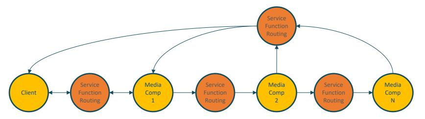
Clients are connected to media functions through frontend routed network, while media functions are chained via service function routing function, the latter being realized as 'fast switching' SDN-based solution
