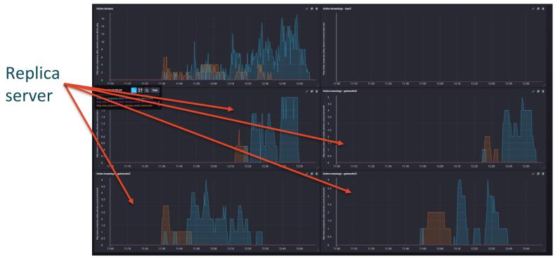
Various streams activated on the different replica serves with direct streaming (blue lines) and transcoding (orange lines)
